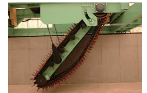
▲ Abrasion-resistant, corrosion resistance special chain
