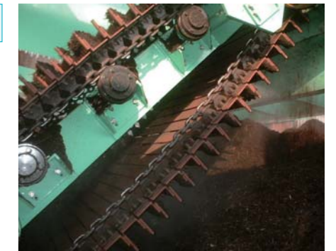
▲ Strong mixing with a scoop style crosscutting device
