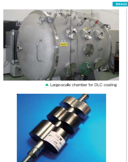
▲ DLC coated vacuum pump rotor
